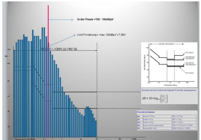
Measured base interference level in public energy supply up to 153dBµV
