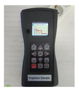
Network Analyzing Handheld NA 02-13 for measuring grid-bound disturbance voltage in the low voltage range, according to EN 55011 - EN 55022 in the range 150KHz – 500KHz and the new Norm CEI – 0-21 for the lower frequency range from 1 KHz to 500KHz
